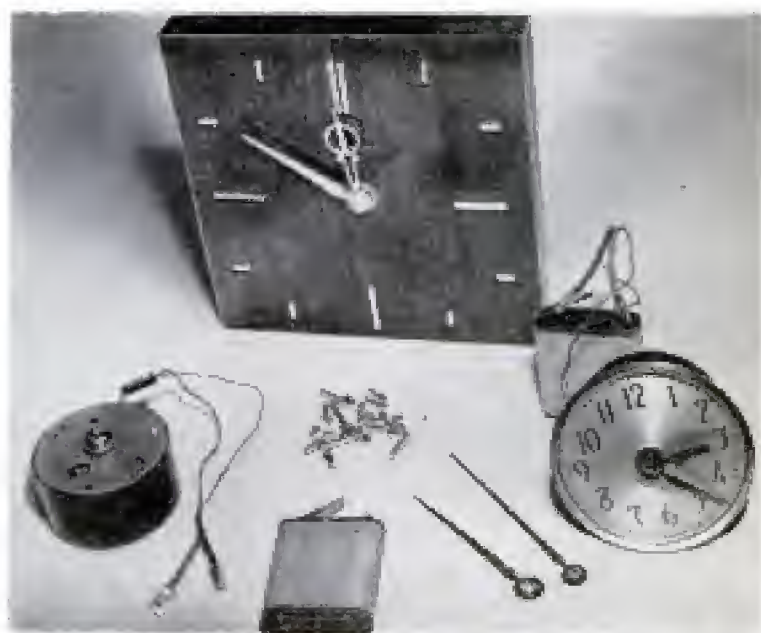
Completed battery-powered clock is in the background, with the kit units in the left foreground. Clock movement and battery are shown at the right assembled as an auto-clock replacement
